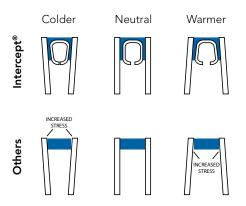
The Blackline spacer features a patented one-piece u-channel design offering superior flexibility with no load on sealant, virtually eliminating seal failure. The unique black coating creates an aesthetically pleasing sight line at the edge of the glass.
